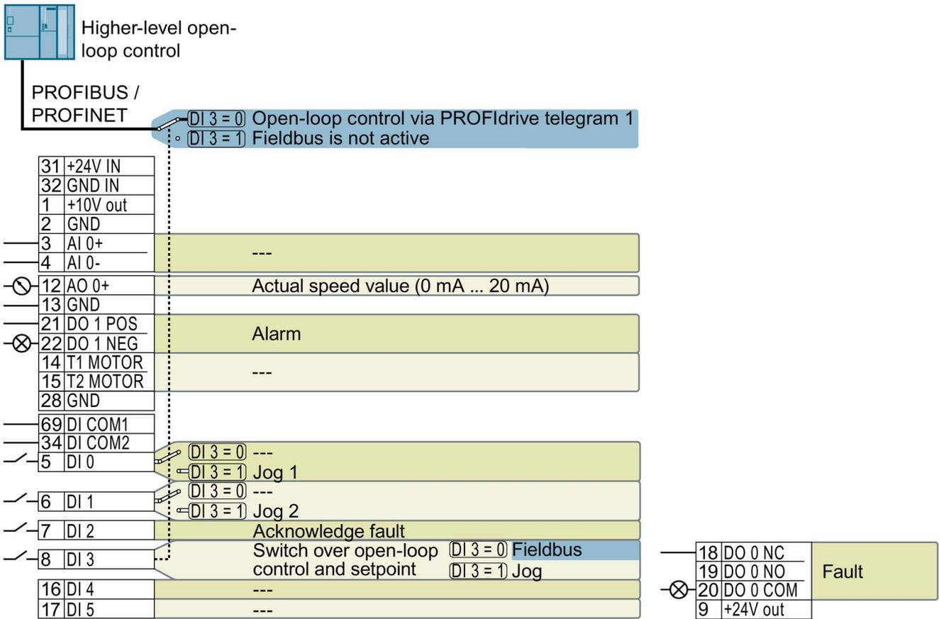
Figure 3-9 Factory setting of the terminals for G120C DP and G120C PN
