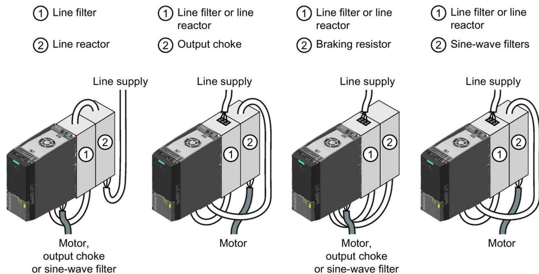
Figure 3-5 Permissible combination of two base components
