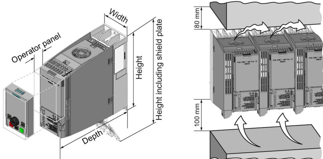
Figure 3-1 Dimensions and minimum spacing to other devices
