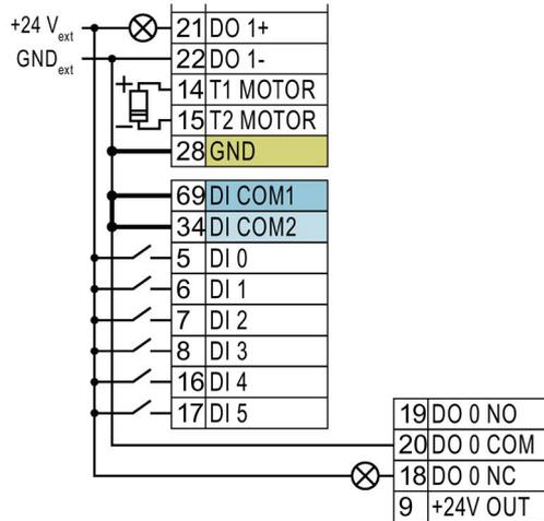
If you want to connect the potential of the external power source to the potential of the inverter's internal power supply, you must connect "GND" to terminals 34 and 69.
