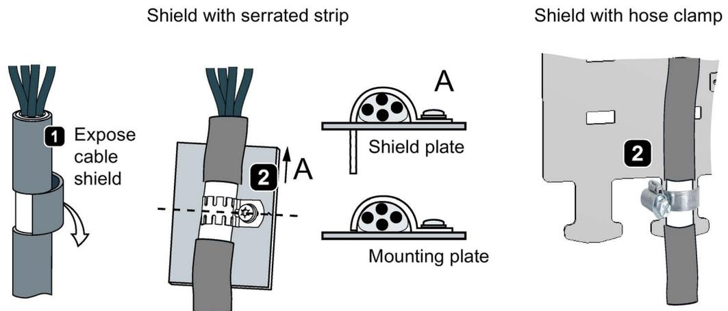
Figure 3-6 Examples of correct EMC-compliant shield connection
