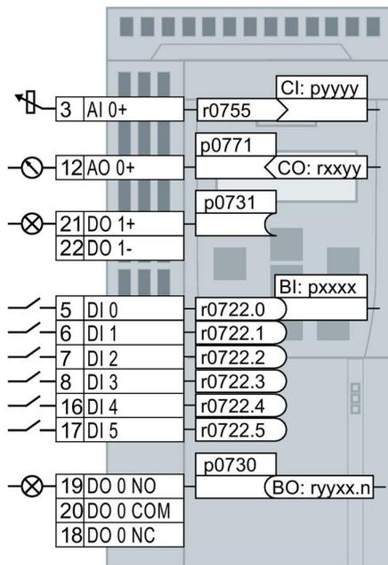
The function of the terminal is defined through a signal interconnection in the inverter:
