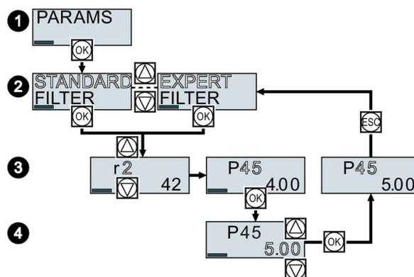
3. Select the required number of a write parameter using the arrow keys. Press the OK key.
