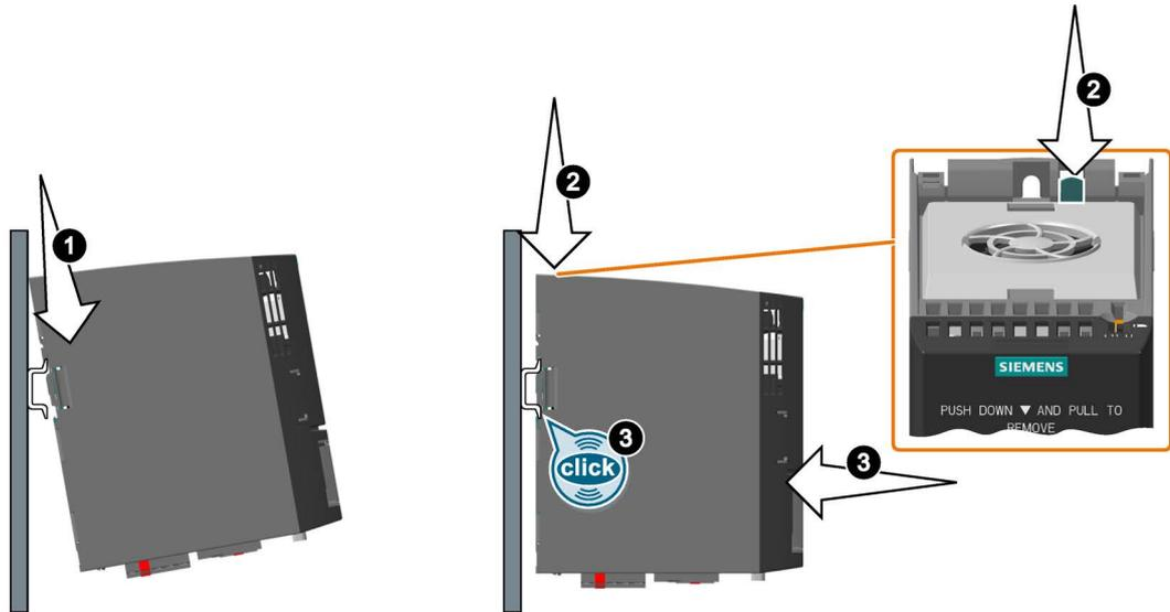
Figure 3-3 Mounting on a standard mounting rail
