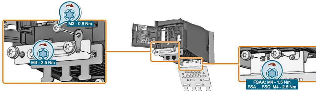
Figure 3-2 Mounting a shield plate using as example a frame size A inverter
